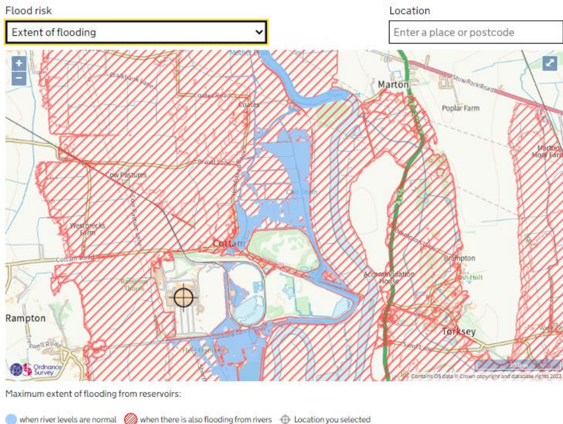
Plate 3: EA extent of reservoir flooding mapping (Ref 13).
